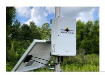
production locations, representing more than 50% of the production in the Haynesville and Marcellus shales. In the Eagle Ford, Chesapeake is piloting a portable methane monitor capable of identifying and quantifying released volumes in real time.
