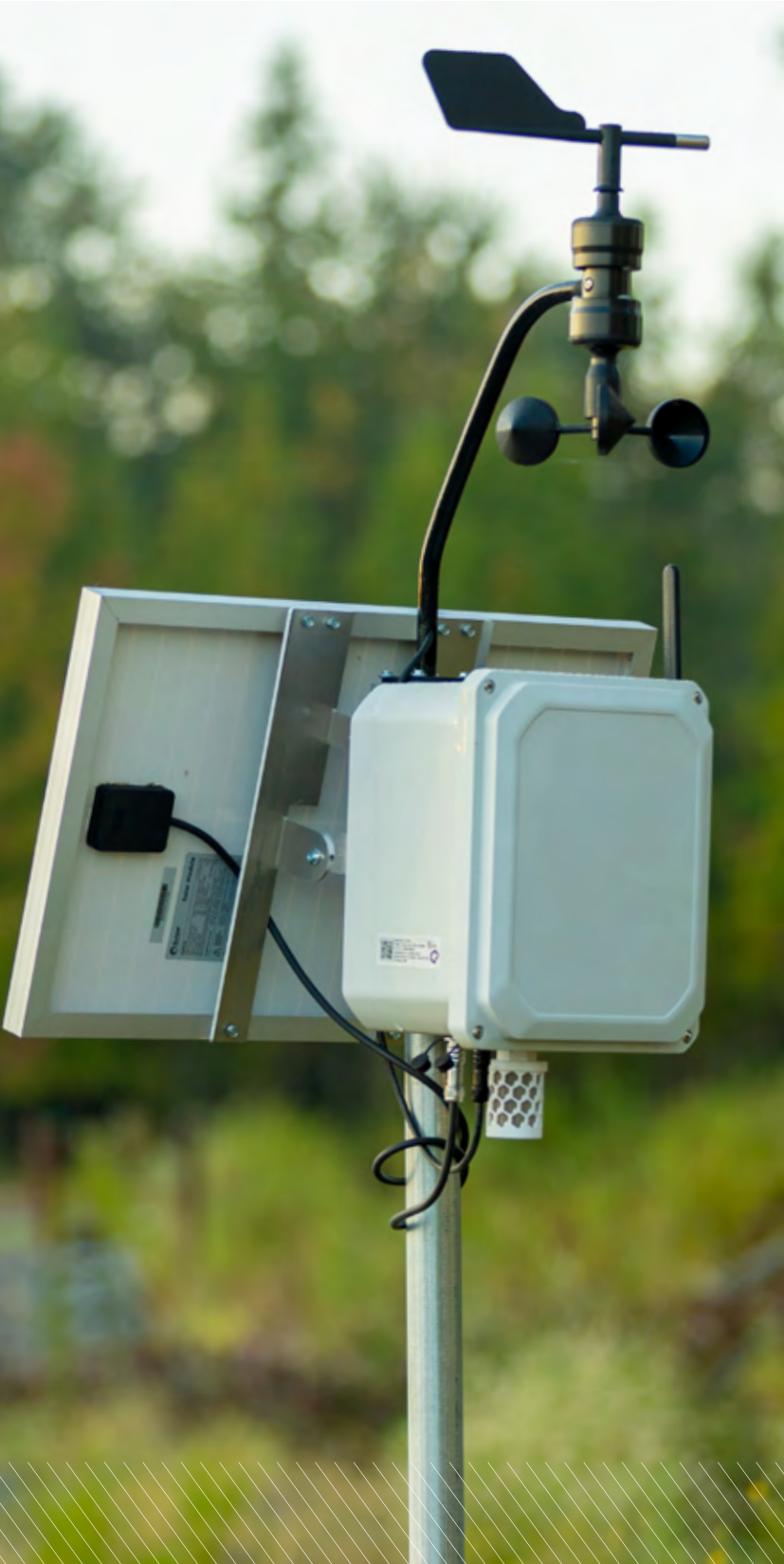
We use fixed monitors for 24/7 detection of methane emissions on our sites.
